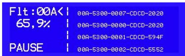
In this window, the complete RDS stream decoded is displayed.
