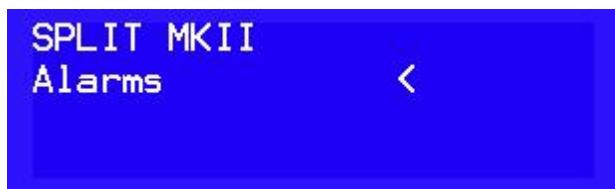
If one or more alarms are active, the front panel **ALRM** led is lit and, into this page, the alarm description is displayed.
