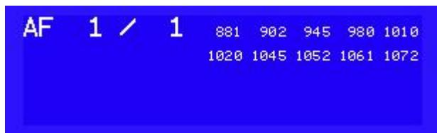
The AF tables being transmitted, are collected and displayed into this window.
