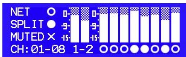
In this window is shown the network input (1-2) level and the output level and status.
