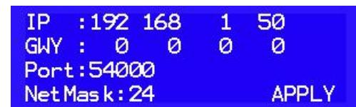
Pressing the knob, an asterisk "\*" will appear next to the first editable element. This will not happen if, on the current window, there are no editable parameters.
