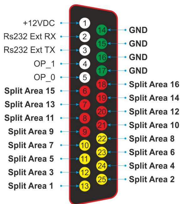
The EXT CNT connector is intended for parallel inputs control.
