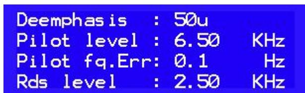
**Deemphasis**      75/50uS/OFF, deemphasis setup for the stereo decoder.
