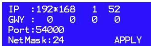
Turn the knob to position the "\*" cursor on the other editable elements of the current window.
