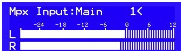
MPX input selection and decoded audio level display.
