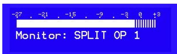
Fine MPX input level monitor for network inputs and splitting outputs,
