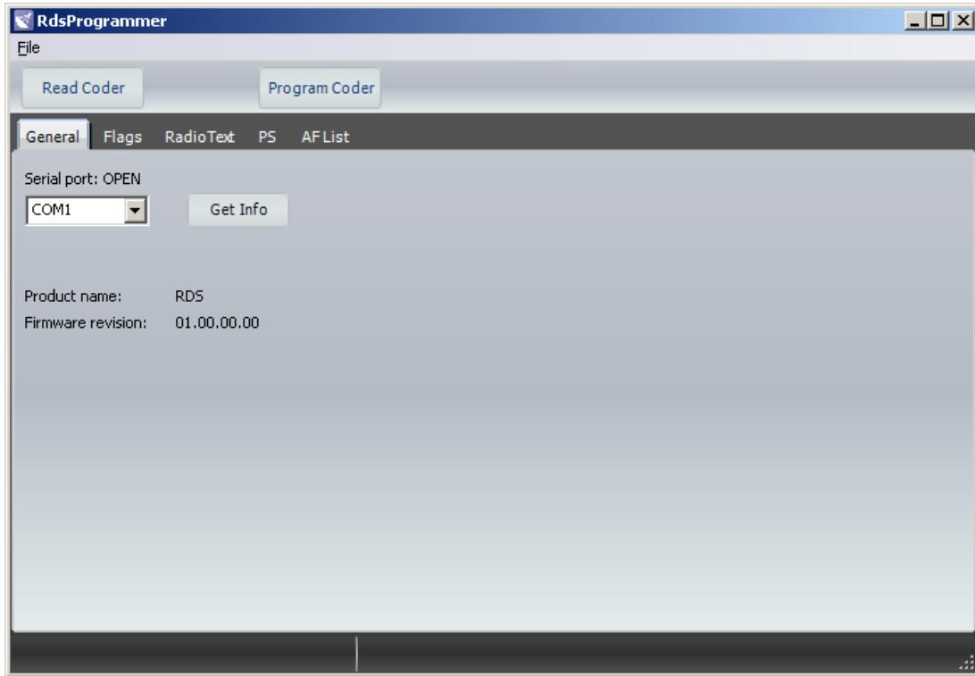
In the main window you can select the COM port used for communication with the RDS encoder
