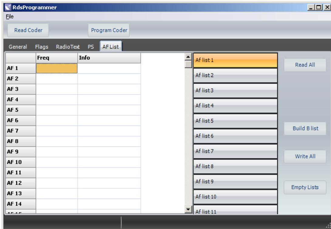
The RDS encoder allows method "A" or "B" for transmitting alternative frequencies.
