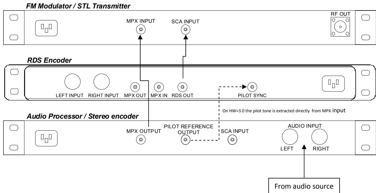
Stereophonic modulation, using external audio processor / stereo encoder and internal RDS mixer.
